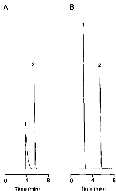
Fig. 2. Chromatogram of pyridine and phenol on the ODS prepared. A=ODS end-capped by liquid-phase silylation (packing No. 24). B=ODS end-capped by HTS (packing No. 6). Peaks: 1=pyridine; 2=phenol.
